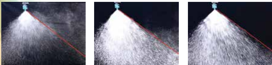
Demonstrates in simulated wind, coarse droplets of: water alone (left), water with glyphosate (center), and water with glyphosate and Leci-Tech (right).
