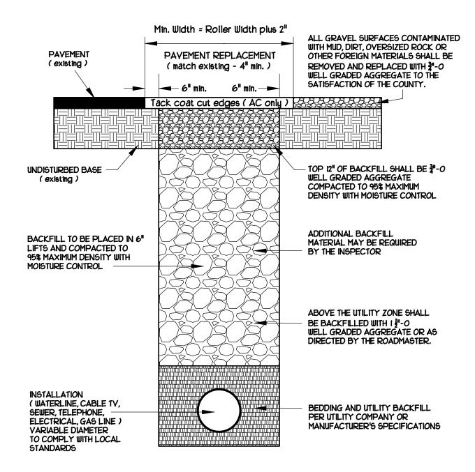
ALL UNDERGROUND INSTALLATIONS SHALL BE BURIED A MINIMUM OF THIRTY (30) INCHES BELOW THE NEAREST VERTICAL ROADWAY SURFACE, (I.E. FROM THE BOTTOM OF THE DITCH LINE). PLANS MUST SHOW THE DISTANCE FROM THE NEAREST VERTICAL ROADWAY SURFACE TO THE TOP OF THE PROPOSED BURIED CABLE, PIPE LINE OR FACILITY.
