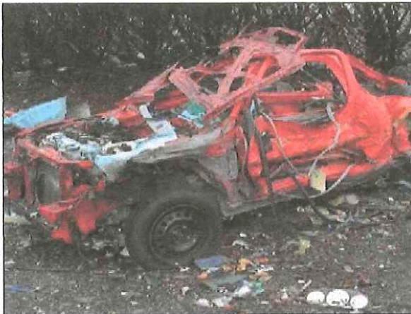
An unconfined vapor cloud explosion at a gasoline storage site in Buncefield, England, in 2005 left bomblike devastation across a wide area. Photo courtesy of the U.K. Health and Safety Laboratory.
