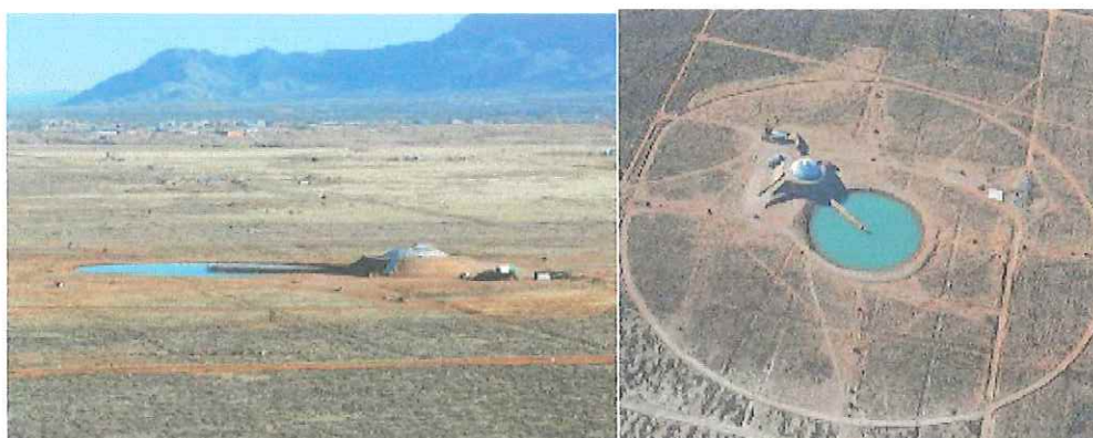
Figure 5. Large-scale LNG pool fire test site.
