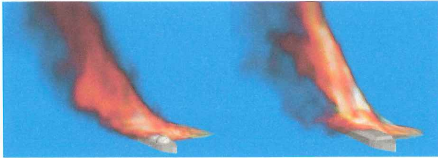
Figure 9. Large pool fire impacts on Moss and Membrane vessels.
