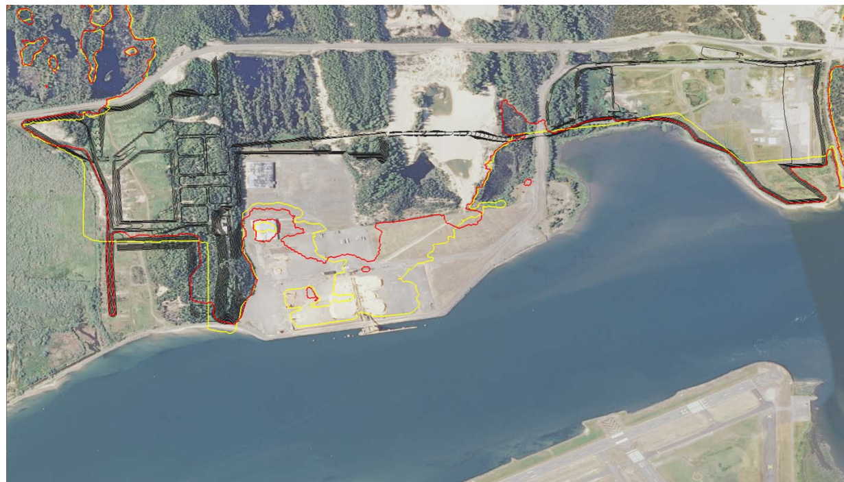
Figure 2. Extent of tsunami wave inundation for L1 Scenario at project site for modified landscape obtained from Zhang (2012) study, shown in yellow and CHE (2013b) study, shown in red
