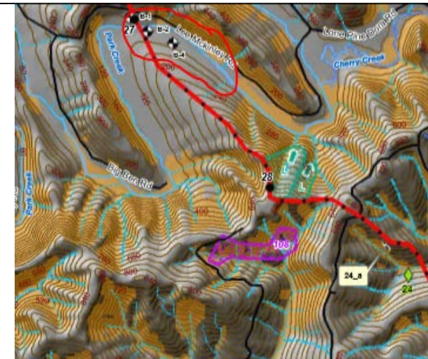
Location of TAR 27.06 near Milepost 27 on the Geologic Hazards Maps. Figure 8 of 47. Note: the light brown areas are Potential Rapidly Moving Landslide Hazard
