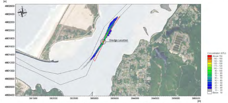
Figure 5-1: Capital dredging with cutter suction dredge, NRI 1
