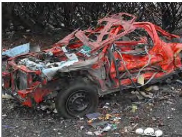
An unconfined vapor cloud explosion at a gasoline storage site in Buncefield, England, in 2005 left bomblike devastation across a wide area. Photo courtesy of the U.K. Health and Safety Laboratory.
