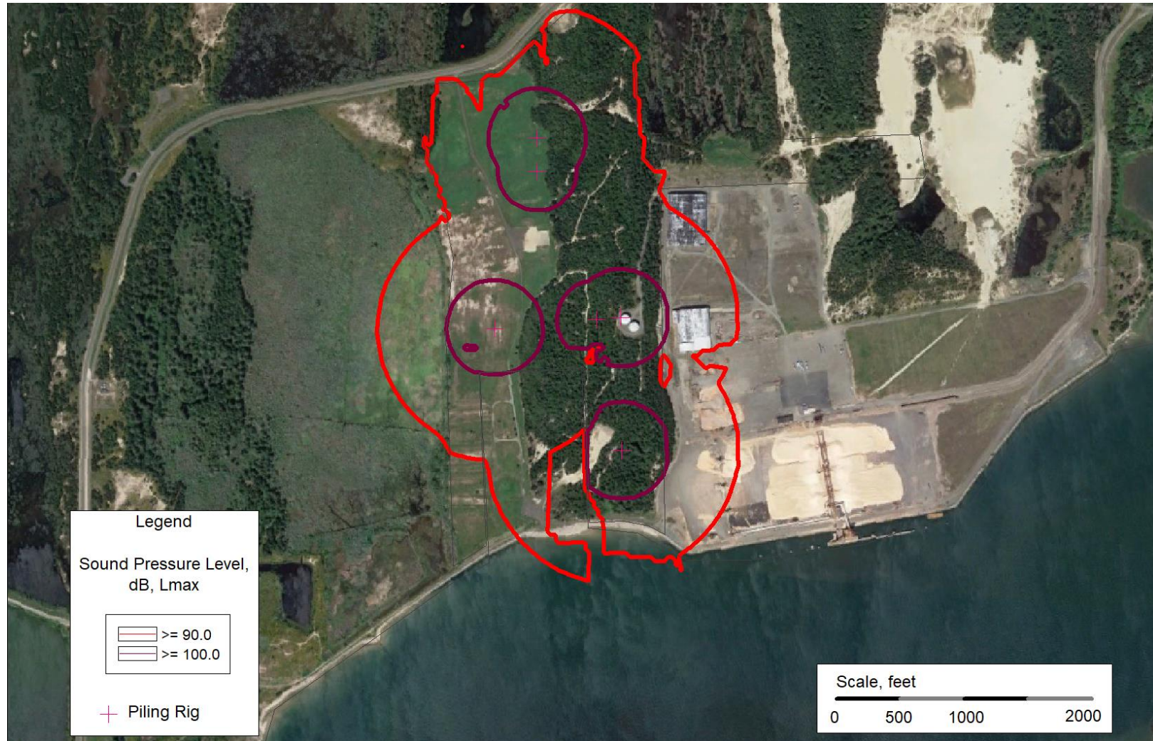
Figure 3 Indicative pile driving in air marine mammal noise impacts
