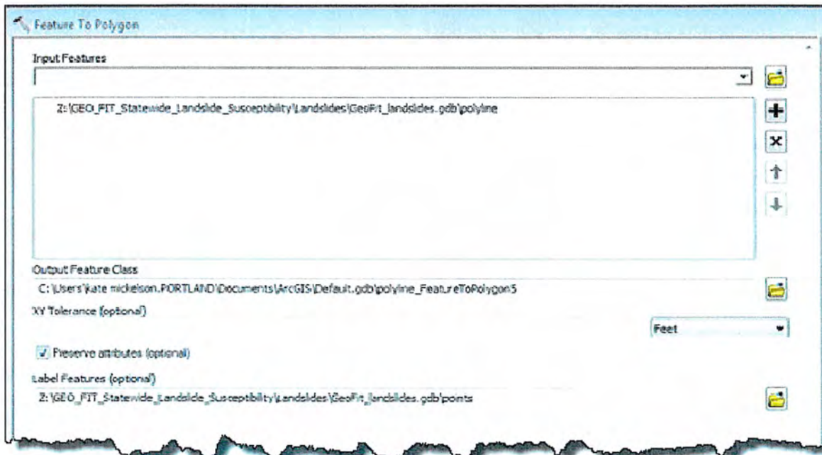
Figure A.2.1. The Esri Feature to Polygon tool is an automated way to remove overlaps in landslide polygons.
