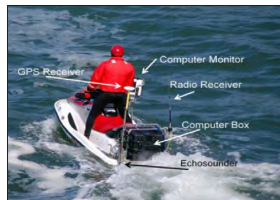
Figure 7. Oregon State University's Coastal Profiling System set-up, which allows access to shallow sections of the estuary. Source: Wood and Ruggiero 2014
