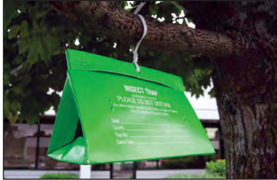
Figure 2. A delta trap, used to detect European and Asian gypsy moths, to facilitate early detection of these species. Source: ODA 2015.
