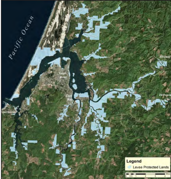
Figure 5. Lands (based on tax lots) that are currently or were historically protected by levees. Data source: OCMP 2011b.
