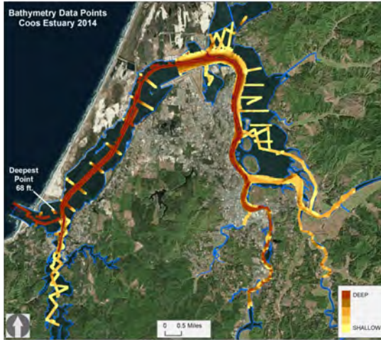
Figure 6. Known bathymetry of the Coos estuary. The estuary boundary is outlined in blue. Data came from regular U.S. Army Corps of Engineer hydrographic surveys, and bathymetry surveying conducted by Oregon State University in 2014. Data Source: USACE 2014; Wood and Ruggiero 2014
