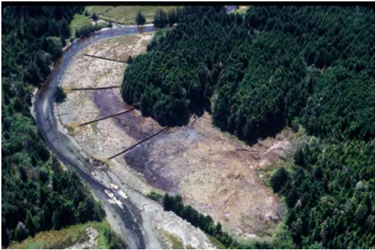
Figure 11. Aerial photo of Kunz Marsh in 1997. The restoration area is divided into four cells by temporary partitions. The elevation of each cell varies with lowest elevation occurring closer to the bottom of the photo and the highest elevation occurring nearer the top. The division of the marsh into cells allowed researchers to examine the effect of marsh elevation on the natural recruitment of emergent salt marsh vegetation and the development of marsh function.
