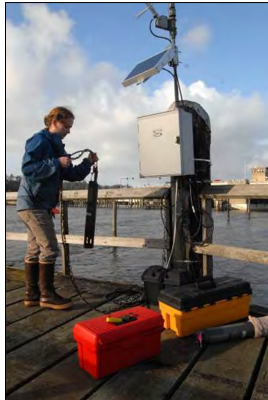
Figure 4. SSNERR staff member deploying a water quality data sonde at the Charleston SWMP station.
