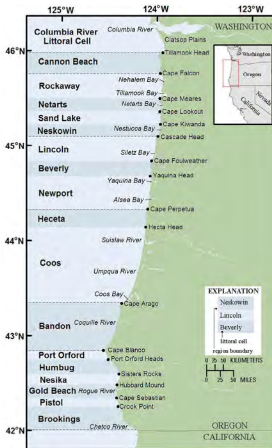
Figure 2. Littoral cells on the Oregon coast (bold text). Cells are stretches of beach bounded by rocky headlands (black dots). Waves transport coastal sediment within each cell.
