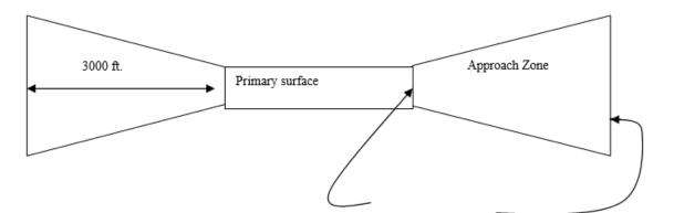
1. Transition Zone – The inner edge of the transition zone coincides with the outer edges of the primary surface and approach zone. The outer edge of the transition zone parallels the primary surface and is 1050 feet wide tapering to the end of the approach zone.
