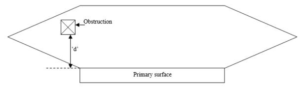
'd' = distance from the primary surface outer edge allowable height =  $(0.14) \times ('d')$  and not to exceed 35 feet.
